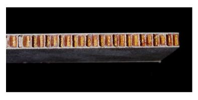
An inner layer of NOMEX(TM) honeycomb, sandwiched between thin G-10 Fiberglass!
