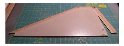
Fiberboard edging provided with kit is glued to the fins using polyurethane glue.
